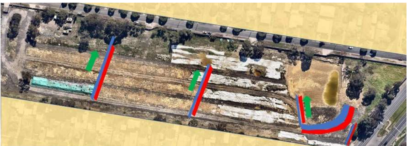
Indicative plan of water drainage works: Blue lines show trenches. Red shows the location of mounds. Green arrows show the fall direction
