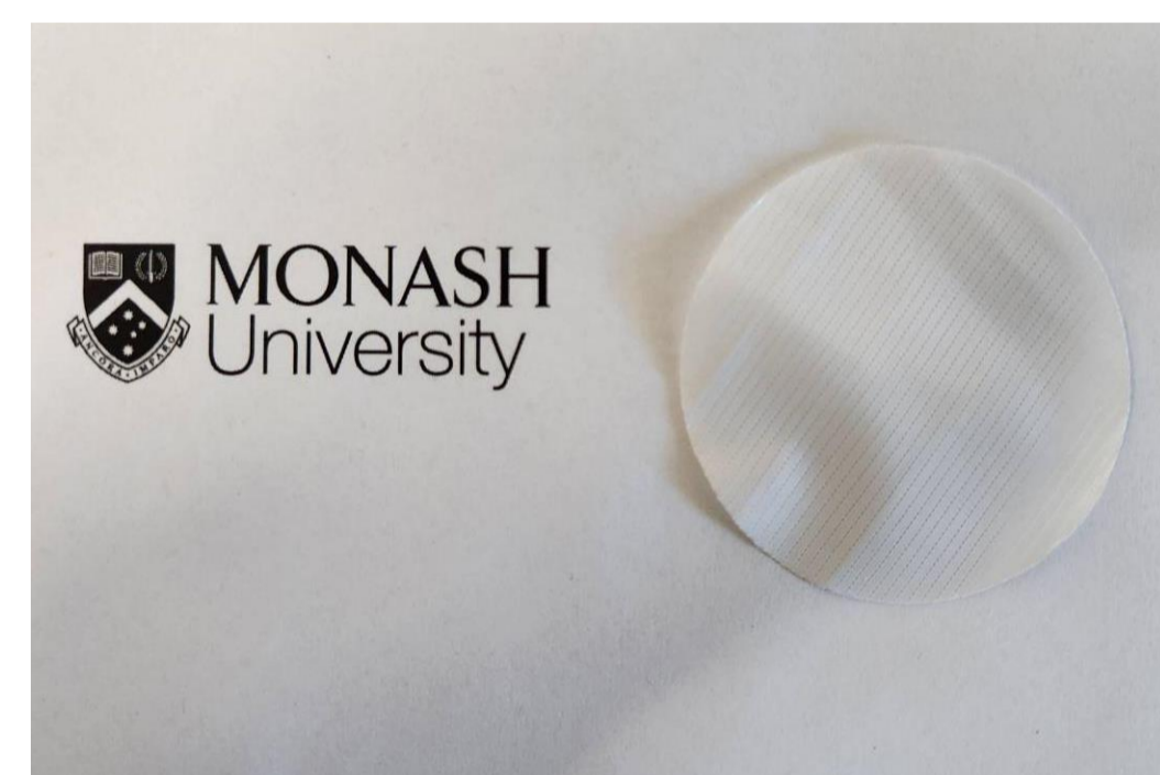
Figure 2: PVA-1 wt.% AlFu-PTFE membrane for ethylene glycol/water separation to allow EG re-use
