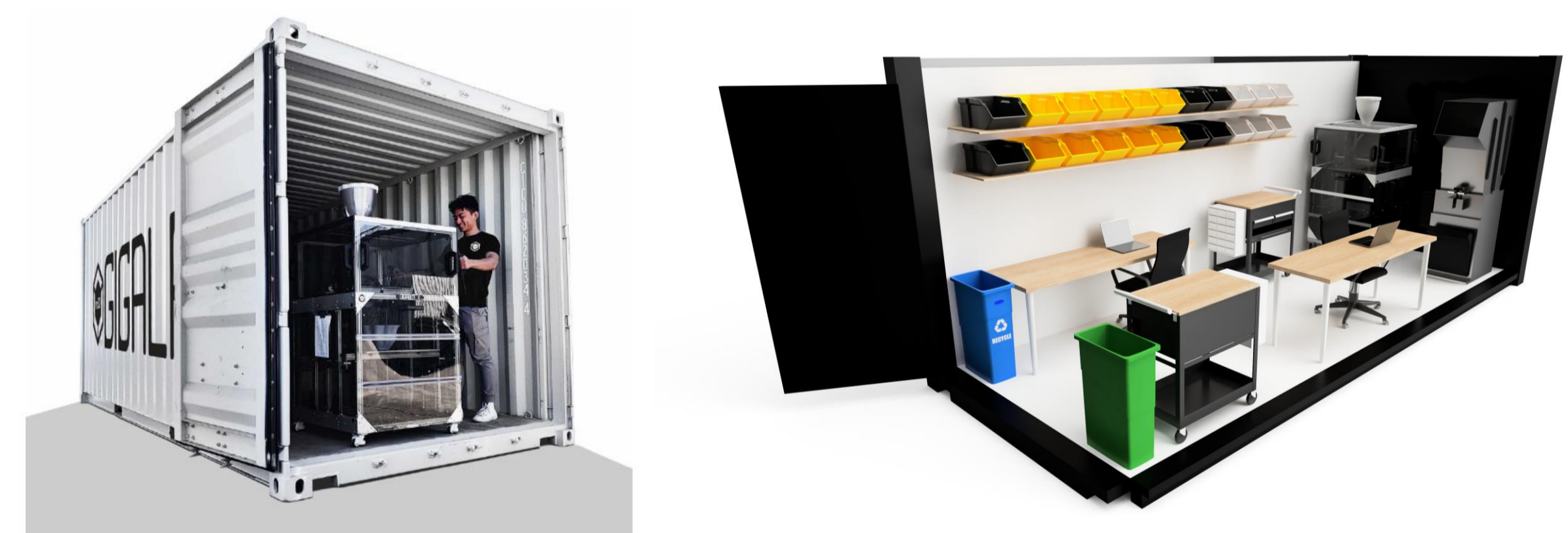
Figure 3: Containerised Gigalab: an all inclusive plastic recycling facility
