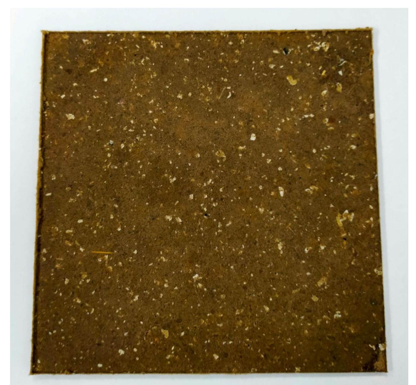
Figure 4: A panel made from post-consumer waxed corrugated cardboard.
