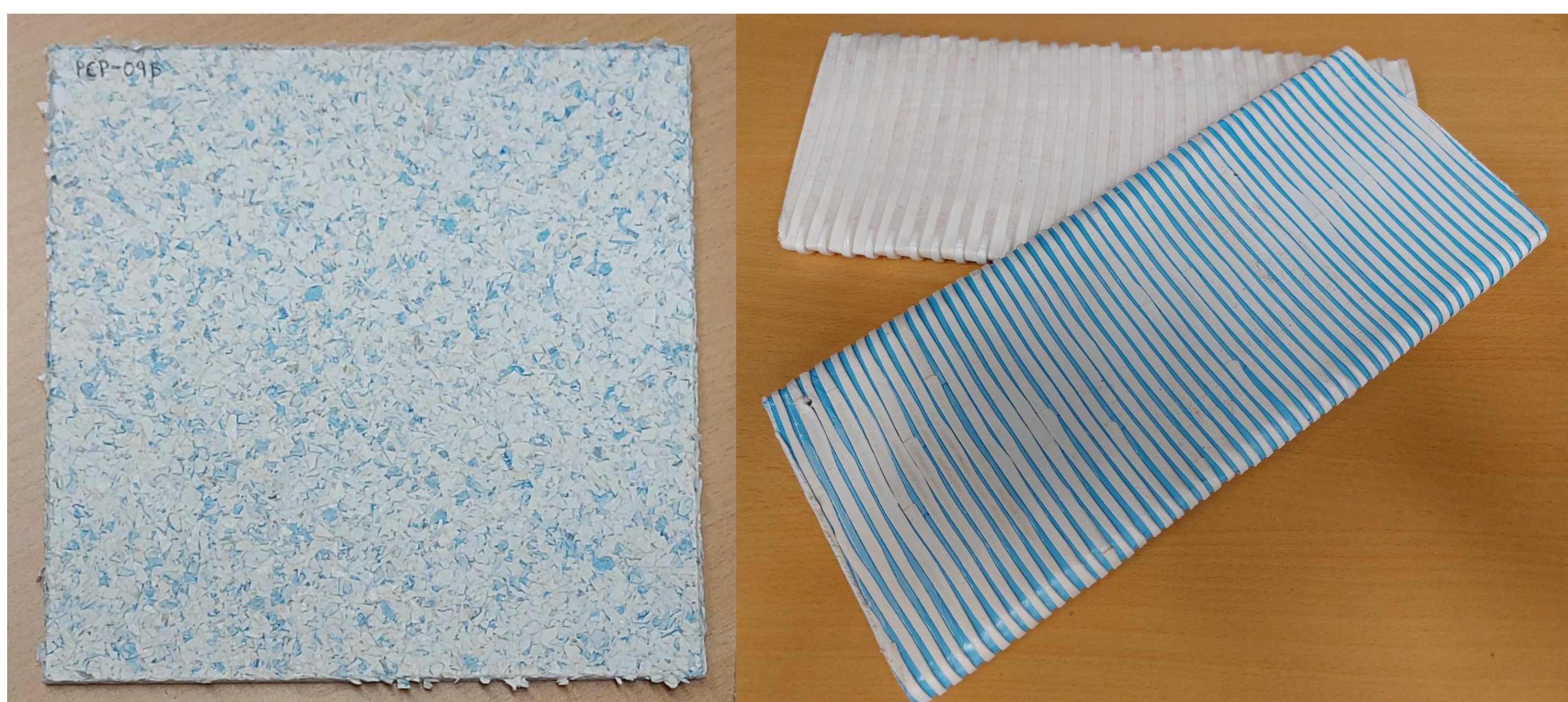
Figure 2: A panel and two boards made from pressing shredded and stacked paper cups, respectively.
