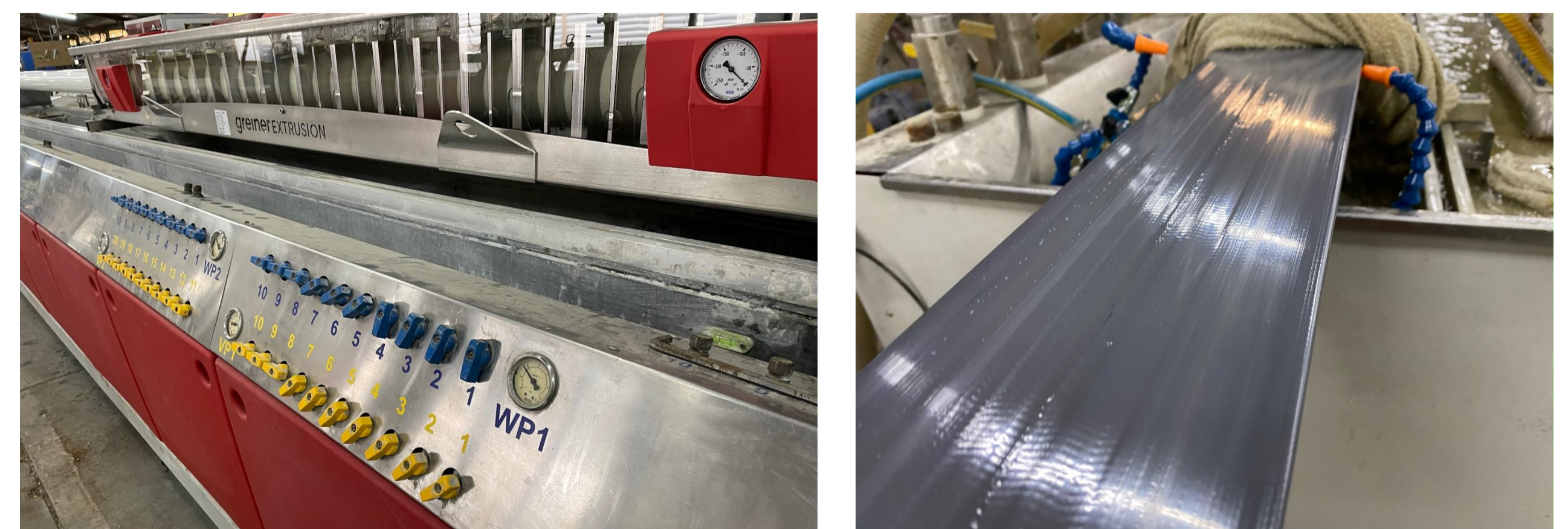
Figure 3: PVC manufacturing process. Photo credits: Think Fencing
