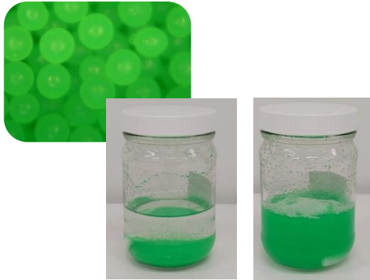
Cospheric PE beads (75-90 \mu\text{m} , 250-300 \mu\text{m} ) in surfactant solution
