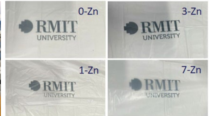
Film blowing and transparency pictures of fabricated composite films
