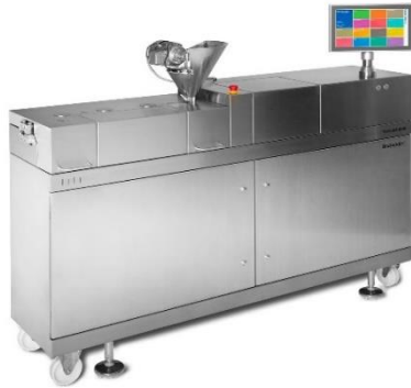
Twin screw extruder TwinLab-F 20/40 + application-specific screws
